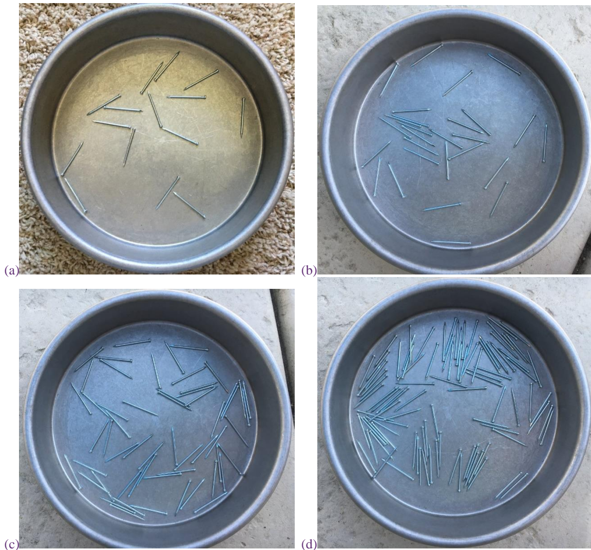
Figure 3.4 Sample configurations after careful “random” shaking: (a) 15 particles. (b) ~27 particles. (c) ~56 particles. (d) ~93 particles.
