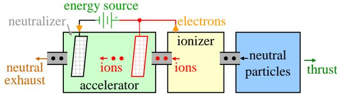
**Figure 2.5:** Ion engine: electric energies are much higher than thermal energies.
