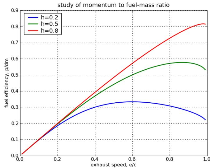
**Figure 2.6:** Some efficiencies of fuel-to-energy conversion in a relativistic rocket.
