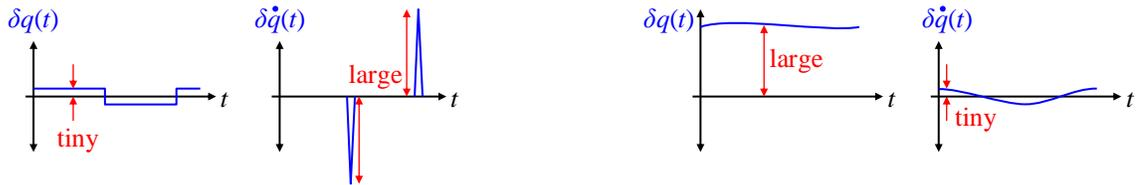
**Figure 5.5** (Left)  $\delta q(t)$  is small, but  $\delta \dot{q}(t)$  is not. (Right)  $\delta \dot{q}(t)$  is small, but  $\delta q(t)$  is not.
