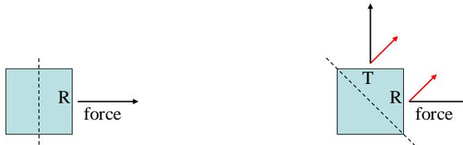
**Figure 4.6** Force on a square tube under pressure: the force along the walls is different than at the corners.
