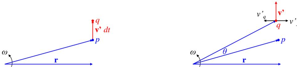
**Figure 3.6** Coriolis acceleration for a tangential velocity. (Left) position of body after  $dt$  is  $q$ . (Right) Velocity vectors at  $q$  after  $dt$ .
