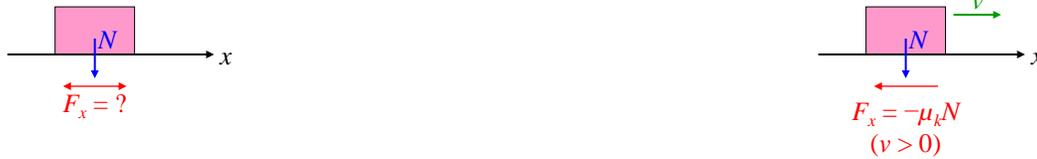
**Figure 4.2** (Left) static friction. (Right) kinetic friction.
