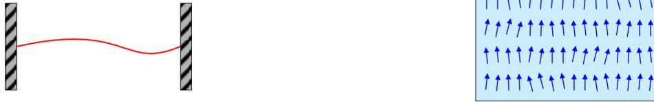
**Figure 5.4** (Left) A vibrating, stretched string has kinetic and potential energy. (Right) Magnetic fields and misalignment of magnetization both store potential energy.
