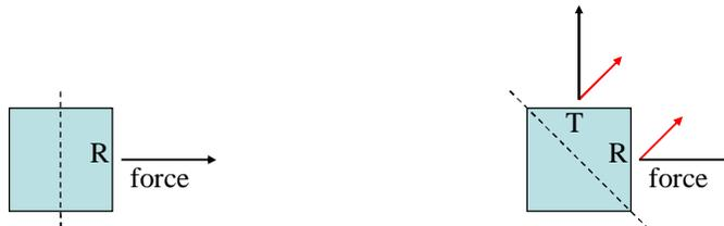
Force on a square tube under pressure: the force along the walls is different than at the corners.
