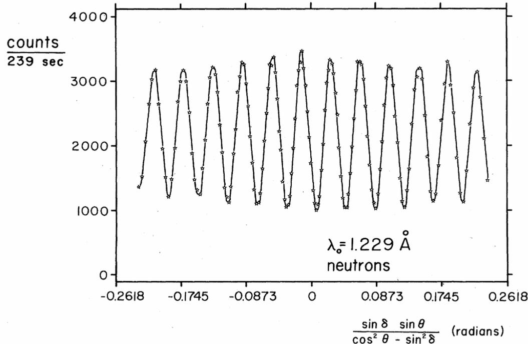
FIG. 7. Example of data obtained by rotating an Si slab in the interferometer (Fig. 6). The counts in detector  $C_3$  are shown.
